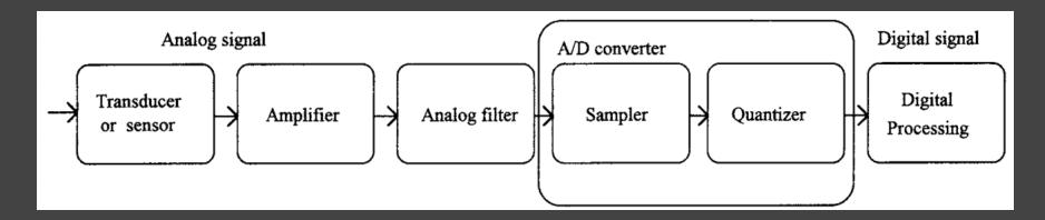
Processing – changing the characteristics of a signal.
