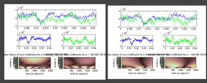
Methods based on continuous wavelet transform (CWT) are used, which can be applied to detection of V-wave in noise signal.
